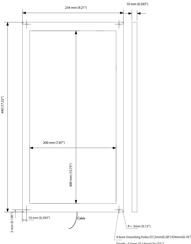
Depth : 3,5mm (0,14mm) for D7,2 5mm (0,20") for D4
